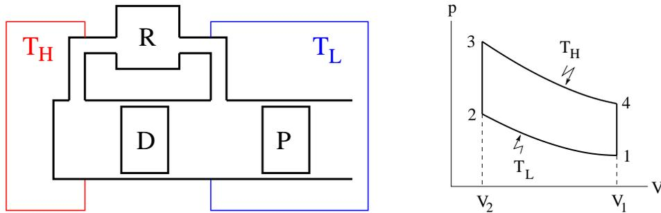
Piston P expands gas at high temperature  $T_H$  and compresses gas at low temperature  $T_L$ .
