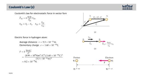
If we wish to express the Coulomb force in vector form as done in the top part of the slide, we must pick one or the other force of the action-reaction pair.  $\vec{F}_{12}$  is the force particle 1 exerts on particle 2. The direction is indicated by the unit vector  $\hat{r}_{12}$  as constructed from the distance vector  $\vec{r}_{12} \doteq \vec{r}_2 - \vec{r}_1$ .
