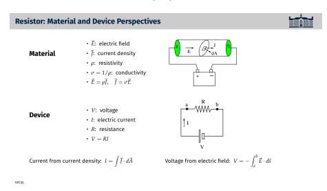
This first slide illustrates the bridge between the material level of description and the device level of description of a steady current driven by a power source.
