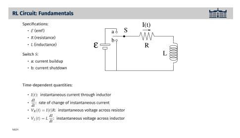
This lecture is devoted to RL circuits, which contain resistors and inductors in addition to EMF sources.
