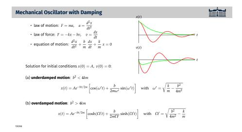
The analogy between mechanical and electromagnetic oscillators still holds in the face of energy dissipation. In the mechanical case we add a damping force to the elastic force [second item]. This adds a term to the differential equation for the function x(t) [third item].
