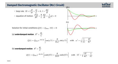
Adding damping to the mechanical oscillator corresponds to adding a resistor to the LC circuit. The mathematical equivalence is quite evident. In the loop rule we now include a term RI.
