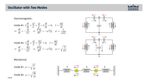
Here we return to an electromagnetic oscillator without damping and its mechanical analogue. The LC circuit with two inductors and three capacitors can oscillate in two different ways (named modes), depending on what the initial state is.
