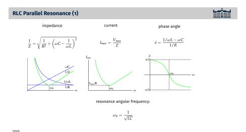
Here we take a closer look at the resonance of the RLC parallel circuit, driven by the EMF  $\mathcal{E}(t) = V_{max} \cos(\omega t)$  with variable angular frequency  $\omega$ .
