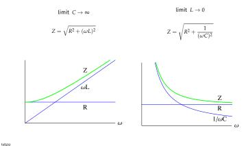
If instead we remove the capacitor from the RLC circuit, we take the limit  $C \to \infty$ . The resulting expression for the impedance of the RL series circuit is shown and plotted on the left. Conversely, removing the inductor, means,
