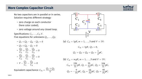
We conclude this lecture with a capacitor circuit that cannot be analyzed by sequential reduction of units that are either series or parallel combinations. The method we use here looks ahead to techniques we shall employ for the analysis of resistor circuits later.
