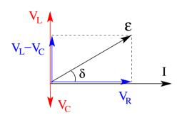
Relation between  $\mathcal{E}_{max}$  and  $I_{max}$  from geometry:
