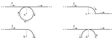
$$B_{a} = \left| \frac{\mu_{0}I}{4\pi R} + \frac{\mu_{0}I}{2R} + \frac{\mu_{0}I}{4\pi R} \right| = |100\text{nT} + 628\text{nT} + 100\text{nT}| = 828\text{nT} \otimes$$
