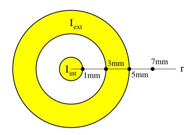
$$2\pi(1\text{mm})B_1 = \mu_0(0.03\text{A}) \quad \Rightarrow B_1 = 6\mu\text{T} \quad \uparrow$$
