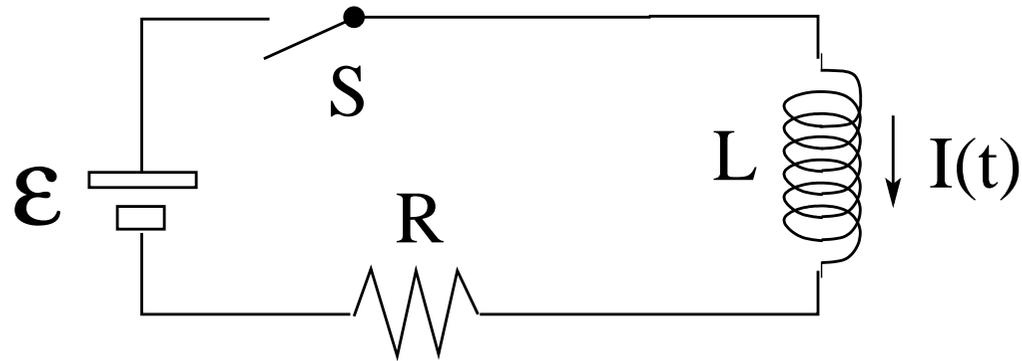
Physical properties of  $RL$  circuit during current buildup determined by 3 combinations of the device properties:
