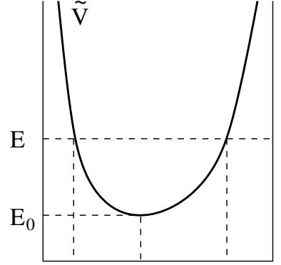
Physical solution for given  $\alpha_{\psi}, \alpha_{\phi}$  requires  $E \geq E_0 = \tilde{V}(\theta_0)$ .
