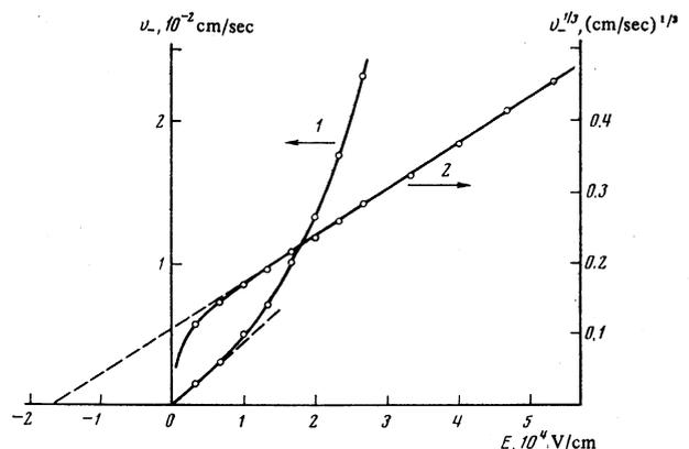
FIG. 1. Typical field dependence of the drift velocity of the charges. Negative charges. Curve 1 (left scale) is shown in a linear scale, curve 2 (right scale)—the dependence of the cube root of the drift velocity on the electric field for the same data;  $p = 36.6$  atm,  $T = 1.43$  K.
