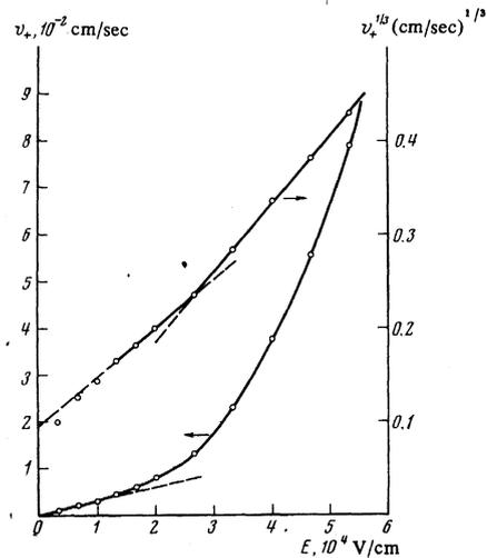
FIG. 3. The lower curve (left scale) gives the dependence of the drift velocity of the charges on the electric field intensity. The upper curve (right scale) gives, for the same data, the plot of  $v^{1/3}(E)$ . The break point corresponds to the electric field intensity  $E_c \approx 2.7 \times 10^4$  V/cm;  $p = 40.5$  atm,  $T = 1.54$  k.
