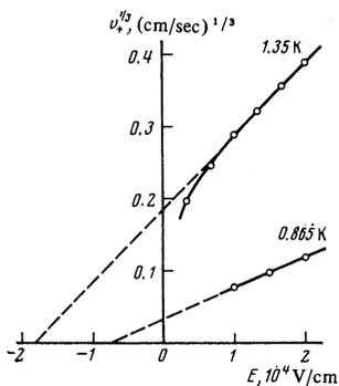
FIG. 2. Plot of  $v^{1/3}(E)$  for different temperatures. The value of field  $-E_0$  corresponds to points of intercept of the straight lines on the abscissa axis:  $p = 32.4$  atm.
