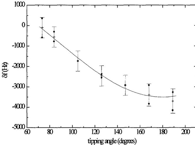
Fig. 4. The variation of the frequency of the signals with tipping angle. The points represent the largest peaks in the spectra while the bars represent the spread of frequencies. The line is a fit to  $\delta f = A(\cos\theta - \cos\theta_c)$ .
