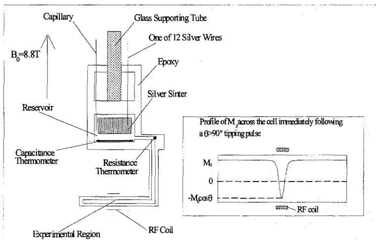
Fig. 1. The experimental cell
