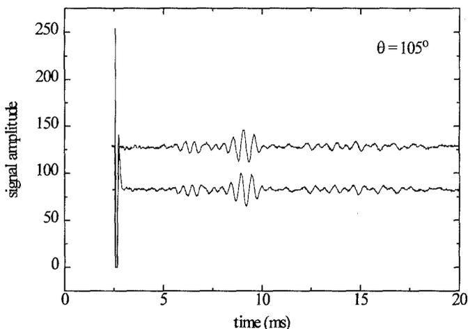
Fig. 2. The in-phase and quadrature signals observed following a  $\theta = 105^\circ$  tipping pulse
